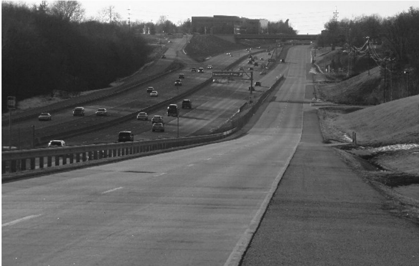
Motorist's view of a one-way frontage road and direct off-ramp from I-64 near St. Louis.
